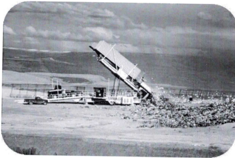
Figure 2-5. Tipping of a Waste Transfer Trailer at the Columbia Ridge Landfill (Source: Seattle Solid Waste Plan - 2011 Revision)
